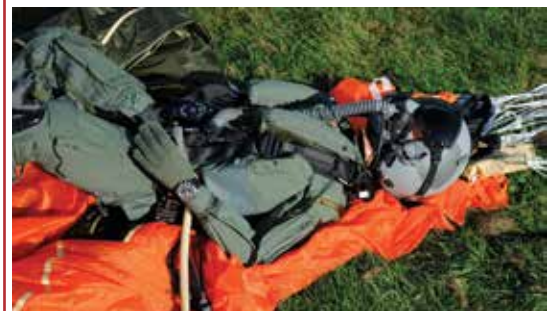
Testing of the MB involved being strapped to the wrist of a crash test dummy and put through a live ejection.
